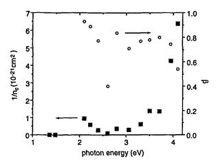
Figure 2: Spectral efficiency of the PPC excitation.  $1/n_c$  and  $\beta$  vs. photon energy.  $1/n_c$  and  $\beta$  is determined by fitting the data from Fig. 1 to Eq. (2).
